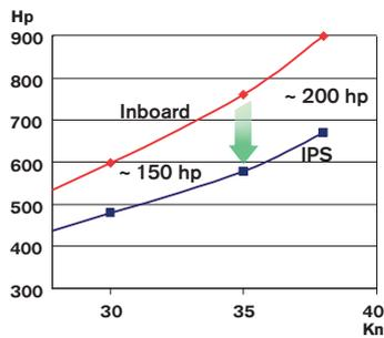
Because of this superior efficiency, the product designations 800/900 communicate engine power required for a conventional shaft installation to reach a comparable performance level.
